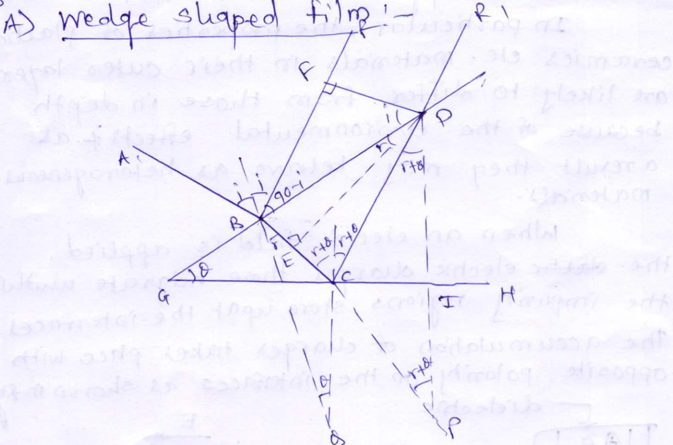
Consider two plane surfaces, GH + GH', inclined at an angle  $\theta$  & enclosing a wedge shaped air film. The thickness of air film increases from G to H as shown in fig.
