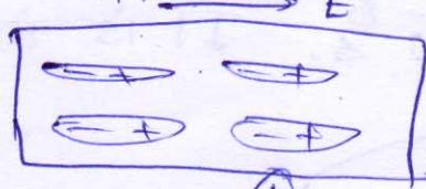
Orientation polarization is characteristic of polar dielectrics, which consists of molecules having permanent dipole moment. In the absence of field the orientation of dipoles is random resulting in a complete cancellation of each other's effect as shown in fig (a)
