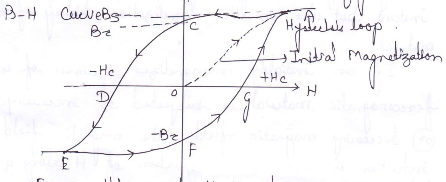
From this graph it is clear that curve decreases rapidly at first indicating big change in the value of  $B$  for a corresponding small change in  $H$ . The slope of the curve gradually decreases indicating a small change in  $B$  for increasing larger values of  $H$ . A stage is reached when the slope of the curve becomes constant and this condition is known as saturation. The units of  $B$  are taken  $\text{Wb/m}^2$  and of  $H$   $\text{AT/m}$ .
