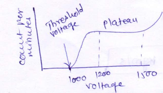
When the voltage is increased secondary ionizat' takes place. Now the no. of impulses increases almost linearly with applied voltage.
